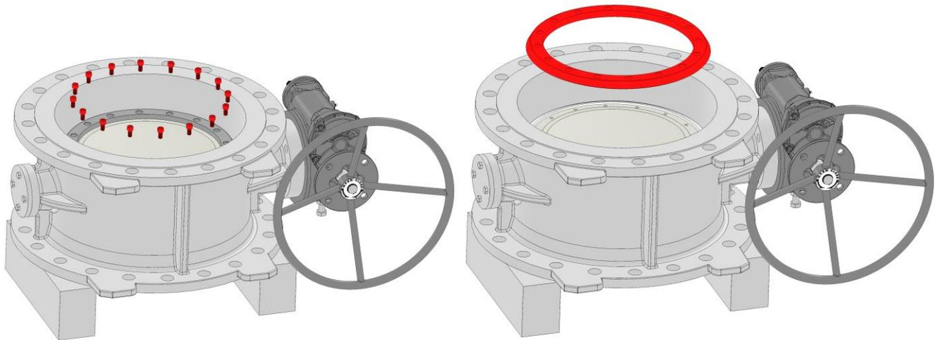
e. Replace the sealing ring with a new one.
