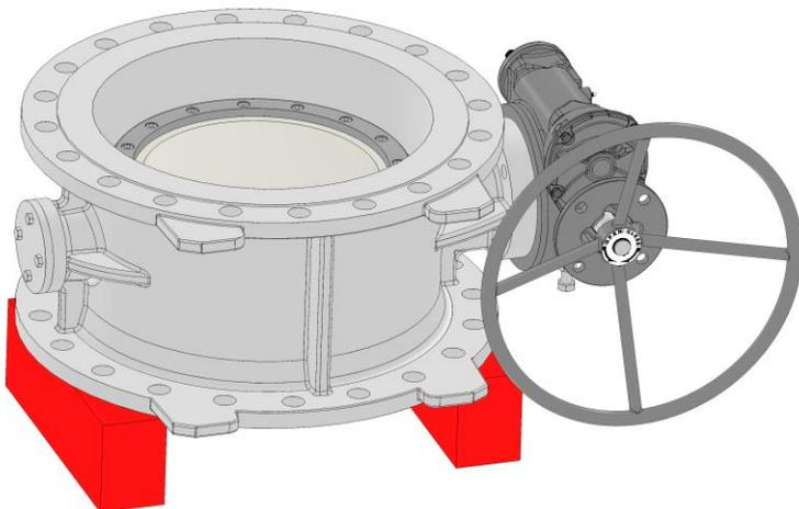
d. Remove the retaining ring bolts and remove the retaining ring.
