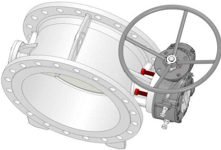
b. Turn the disc 180° by rotating the gearbox.
